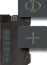
Step 1 - Press the function button for 1s to enter programming mode - to be discovered.
